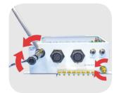
When tightening power lug use wrench to secure backing nut and torque main nut to 105 in/lbs.
